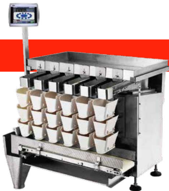
6H4G1.5A-AS 6 Heads anti-sticky weigher (Conveyor feeder)
